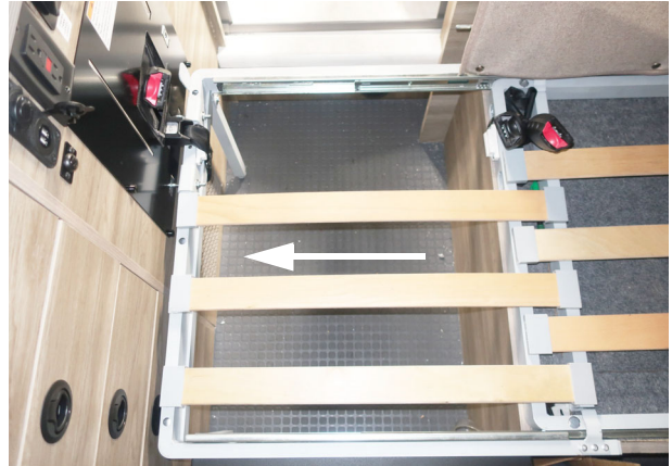
Lift up the seat cushions and slide the other bed support bracket to the extended position. - Typical View
