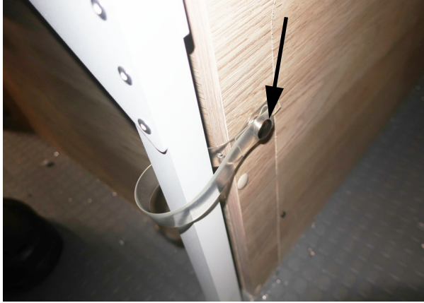
Unsnap the seat retention strap on the rear seat. - Typical View
