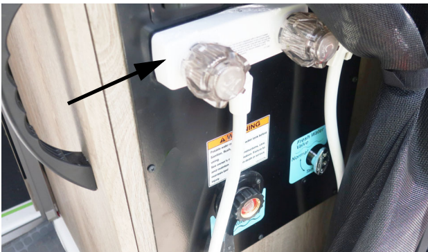
Wash Station (located behind rear passenger door. Lift hinged cover to access) - Typical View
