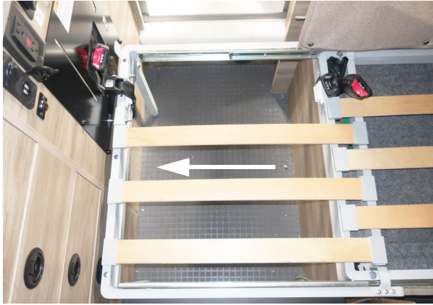
Lift up the seat cushions and slide the lower support bracket to the extended position. - Typical View
