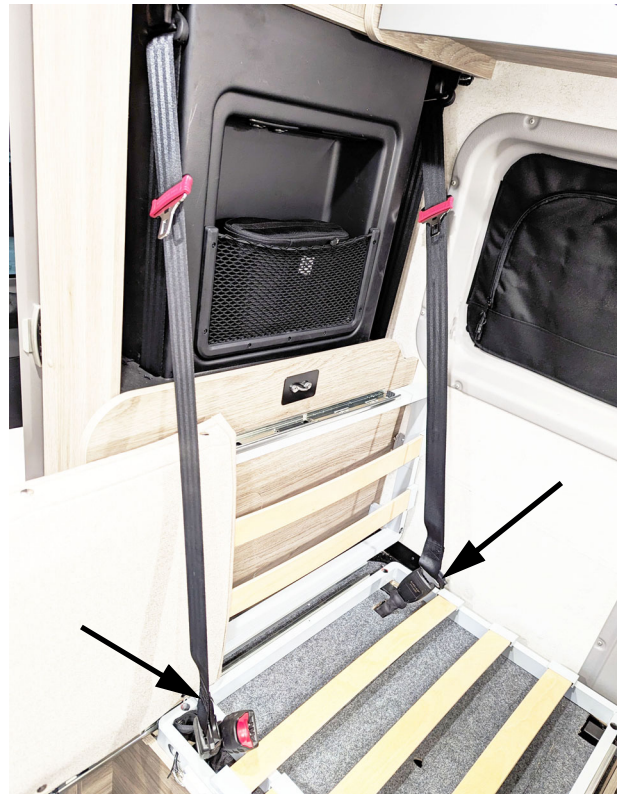
The seat belts are pulled from the ceiling and attached at anchor points shown above. Now these are ready to be pulled across in the seat as a 3 point style seat belt. - Typical View
