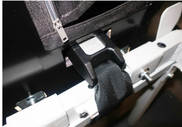
Lower retaining belt shown secure. - Typical View
