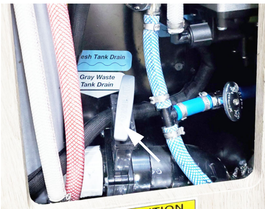
Gray waste tank drain valve (shown closed- pull lever out to drain) T36B shown. - Typical View
