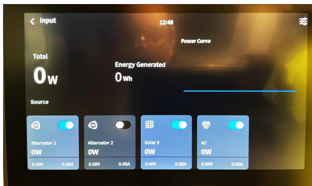
The input screen shows total charging power in Watts, energy generated in watt-hours, and accesses controls of the 2 alternators, Solar and AC shore power. -Typical View
