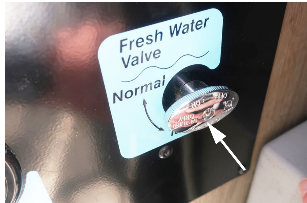
Fresh Water drain Valve (Located on Water Center Panel shown in the closed position for the T36A and T36B). -Typical View
