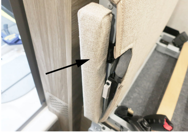
Remove the upper seat pad from the seat and seat back to expose the insertion pins. - Typical View
