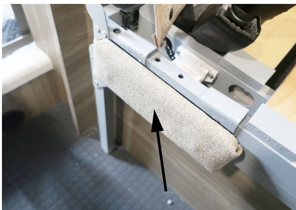
Remove the lower seat pad from the seat and seat back to expose the insertion pins. - Typical View
