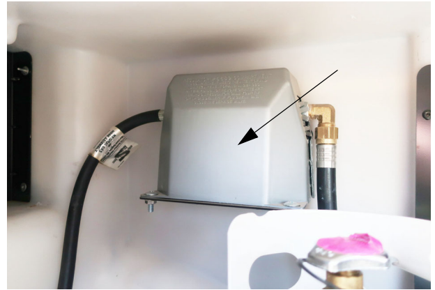
Propane Gas Pressure Regulator- Located on the back wall of the LP access compartment. -Typical View
