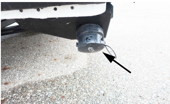
Sewage Drain Outlet (Located beneath the motorhome on the driver side rear.) - Typical view
