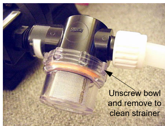
Water Pump Strainer -Typical View
