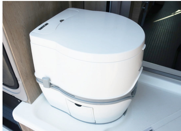
Cassette Toilet. (T36B Shown- T36A is located underneath rearward facing dinette seat.) -Typical View
