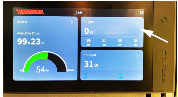
On the home screen, tap the screen inside the input box to open the input control panel. -Typical View
