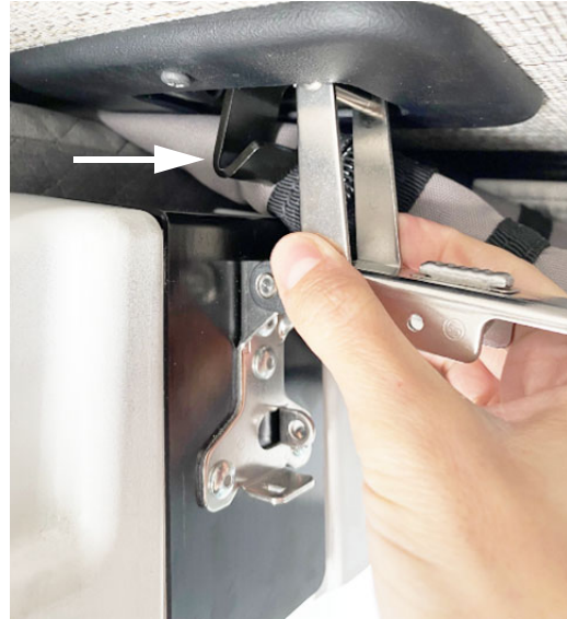
Travel latch retaining hook. -Typical View
