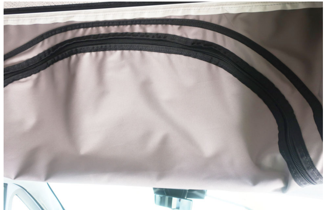
When pulling the pop-top down, pull the fabric in to avoid pinching it in the pop-top. This will make it easier to latch and will help avoid any damage. -Typical View
