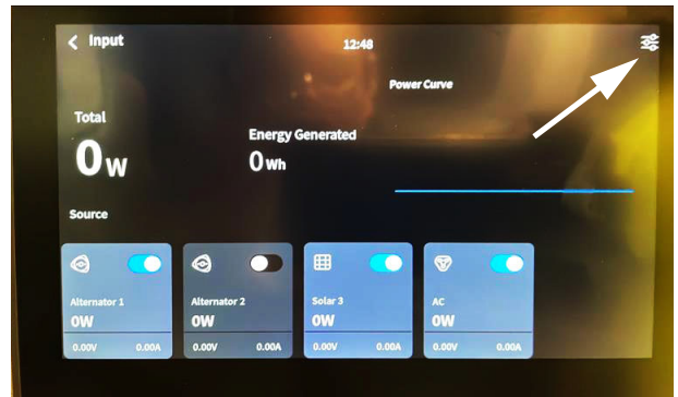
While on the input control panel screen, tap the settings bar icon in the upper right hand corner to open the input setting screen. -Typical View
